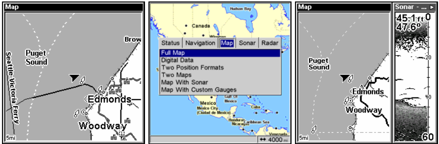
Full Map page (left). Pages Menu with the Map option list (center). The Map with Sonar screen (right).
